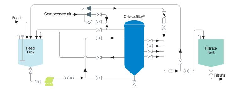
The cocoa powder is separated into a cone by sedimentation. And the cake that is left is deposited at the bottom of the vessel before being reintroduced into the tank.
