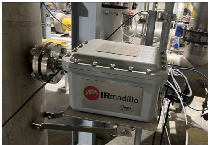
The IRmadillo installed in an ethanol fermenter recirculation line at Elite Octane
